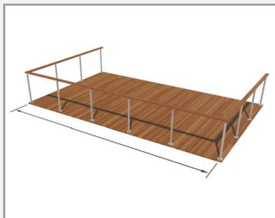
Mark out and drill all posts at the required spacing and hole size. Flip toggle end post 6mm (inside face only), hex head tensioner post 9mm outside face, 7.5mm inside face and intermediate posts 7.5mm.
