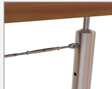
Reattach all the fittings to the rigging screw and attach to saddle on opposite end. Tension the wires with your ProRig c-spanner by rotating the rigging screw as shown.
