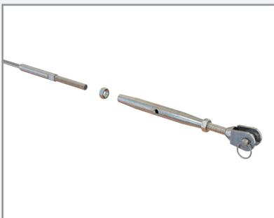
Remove the rigging screw and nut from the opposite end of your wire, this will allow you to pass your wires through the pre-drilled 7.5mm holes in your intermediate posts.
