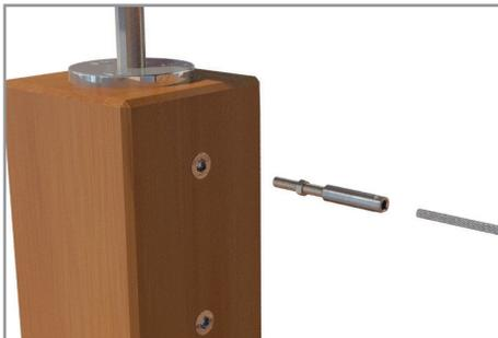
Firmly push the wire into the opening of the right hand threaded Rapid Lock Swageless Stud so that contact with the internal back end can be felt. Rapid Lock's patented one-way jaw system will lock the wire in place.
