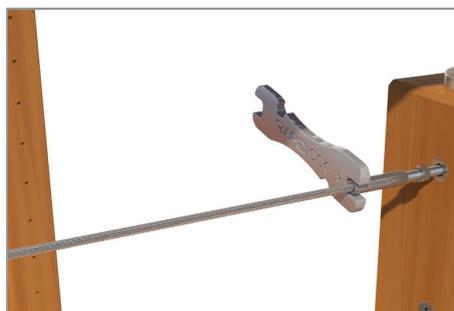
Wind the left hand Rapid Lock stud anticlockwise into the left hand threaded insert, and take note that the other end is rotating and tensioning at the same rate. Continue to wind by hand until the wire is mostly tensioned, then complete using the Rapid Lock Multi Tool.
