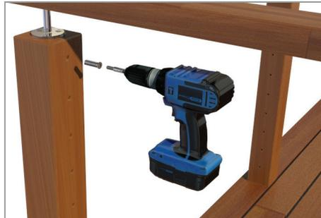
Use the 6.4mm hex drive bit to screw the threaded inserts into the pre-drilled end posts. Note: Insert all left hand threaded inserts into left hand post and all right hand threaded inserts into right hand post.
