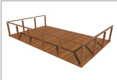
Mark out and drill all posts at the required spacing and hole size of 7.5mm. It is recommended that holes in the end posts be drilled 40-50mm deep and then countersink for a neat finish.
