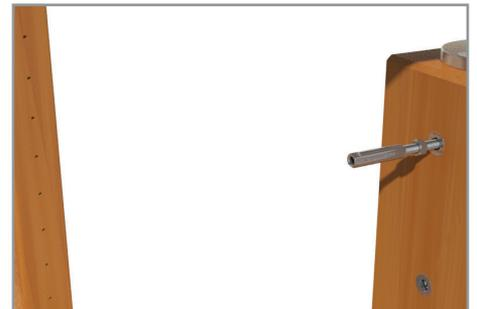
At the other end thread the left hand threaded Rapid Lock Stud anticlockwise into the left hand threaded insert. Rotate 2 full turns.
