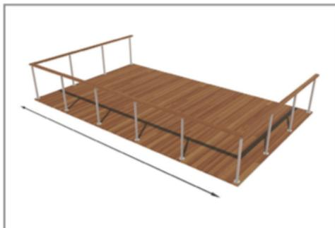
Mark out and drill all of your posts at the required spacing and hole size. This system requires a 10mm hole in end posts and at least a 4mm hole in the intermediate posts.
