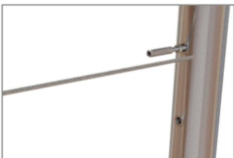
Pull the wire tight and hold against the body of the left hand threaded Rapid Lock stud. Cut the wire in line with the edge of the stud where the thread starts. Firmly push the wire into the opening of the left hand threaded Rapid Lock Swageless Stud.
