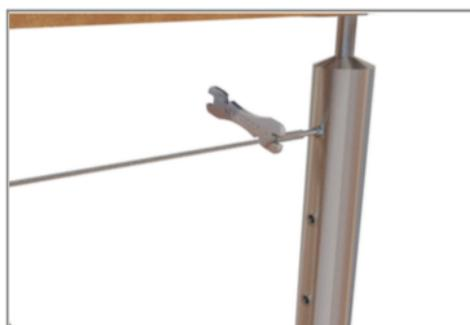
Thread the right hand threaded Rapid Lock Stud clockwise into the right hand threaded insert. Rotate 2 full turns.
