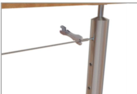
Wind the left hand Rapid Lock stud anticlockwise into the left hand threaded insert, and take note that the other end is rotating and tensioning at the same rate. Continue to wind by hand until the wire is mostly tensioned, then complete using the Rapid Lock Multi Tool.
