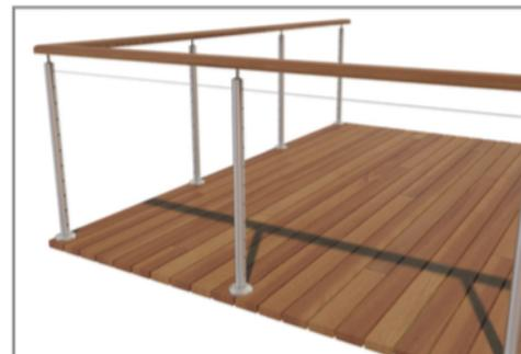
Pass the wire through any pre-drilled intermediate posts.
