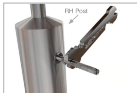
At the other end thread the left hand threaded Rapid Lock Stud anticlockwise into the left hand threaded nutsert. Rotate 2 full turns.
