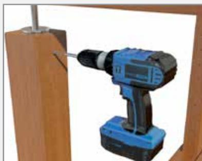
Pre-thread pre-drilled holes with left and right hand lag screws (order separately). Ensure right hand threaded lag screw is used on the right hand side end post and left hand threaded lag screw is used on opposite post.
