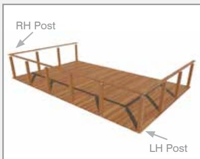
Mark out and drill all posts at the required spacing and hole size (end posts 4mm, intermediate posts 7.5mm). The depth of the hole should be 45-50mm deep.
