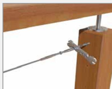
Reattach all the fittings to the rigging screw and tension the wires with your ProRig c-spanner by rotating the rigging screw body.
