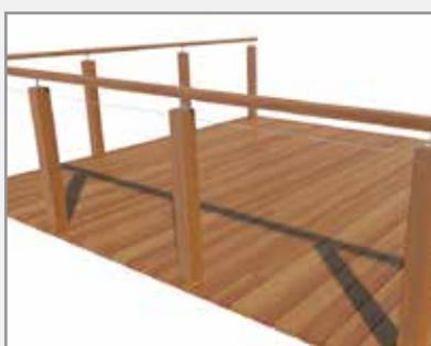
Pass the opposite end of the wire through the pre-drilled intermediate posts. Ensure the body and nut of the rigging screw are taken off before attempting to pass the wire through.
