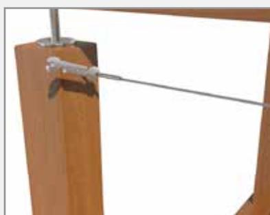
Screw the right hand threaded lag screw in using the ProRig c-spanner until the entire thread is embedded in the end post.
