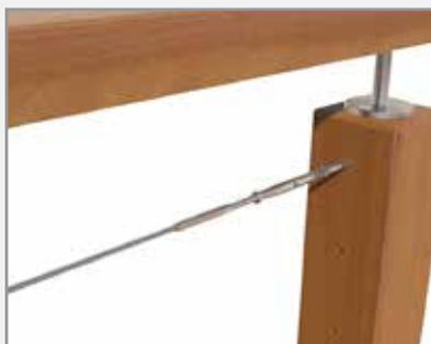
Lock the hex nuts against the body of the rigging screw to lock the system in place.
