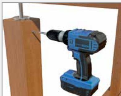
With the right hand lag screw provided pre-thread the pre-drilled holes in the end post (one end only).
