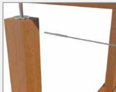
Screw the right hand threaded lag screw into the pre-threaded hole.
