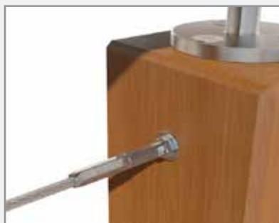
Once the desired tension has been achieved, lock the system in place by tightening the hex nuts against the head of the threaded inserts.
