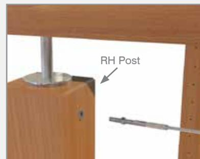
Make sure the right hand swage stud is wound into the right hand threaded insert, only screw the swage stud into the threaded insert the minimum amount possible for wire to hold.
