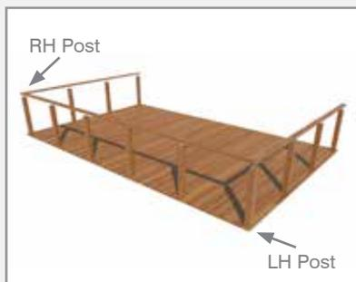
Mark out and drill all posts at the required spacing and hole size of 7.5mm. It is recommended that holes in the end posts be drilled 40-50mm deep and that the hole is countersunk to prevent splitting.
