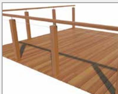
Pass the opposite end of the wire through the pre-drilled intermediate posts (remove nut before passing swage stud through).
