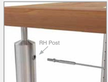
Make sure the right hand swage stud is wound into the right hand nutsert, only screw the swage stud into the nutsert the minimum amount possible for wire to hold.
