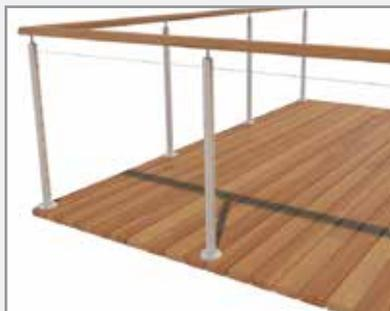
Pass the opposite end of the wire through the pre-drilled intermediate post (remove nut before passing swage stud through).
