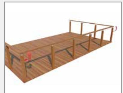
Tighten both ends evenly by rotating the wire in the same direction using the ProRig c-spanner.
