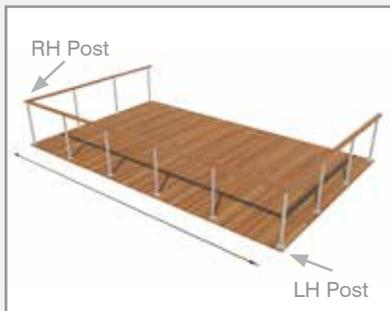
Mark out and drill all posts at the required spacing and hole size (end post 10mm, intermediate 7.5mm). **Note:** ProRail posts can be supplied with all holes pre-drilled.
