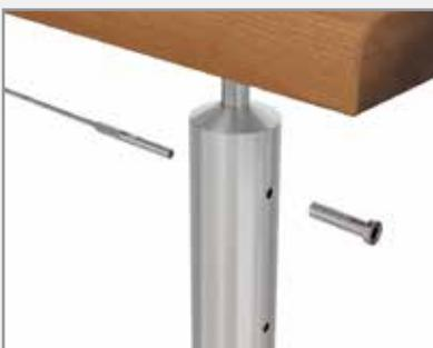
Insert the hex head tensioner into the 9mm hole on the outside face of the post. Thread the tensioner onto the swage stud. (threads will meet inside the post).
