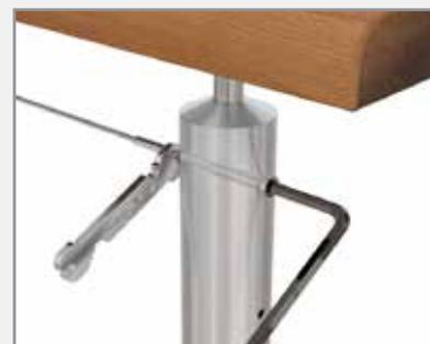
Using a ProRig c-spanner hold the swage stud, using a 1/4" allen key tighten the hex head tensioner until the desired tension is achieved.
