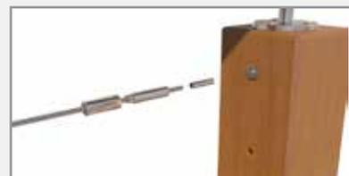
On the open end of the wire thread the finishing cap, tension rod & swage terminal (as above). Crimp the swage terminal four times.
