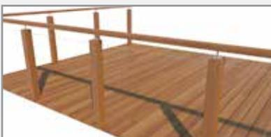
Pass the opposite end of the wire through the pre-drilled intermediate posts.
