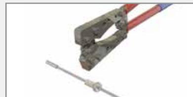
Crimp the swage terminal four times using the HX-50 swage tool (setting 6).
