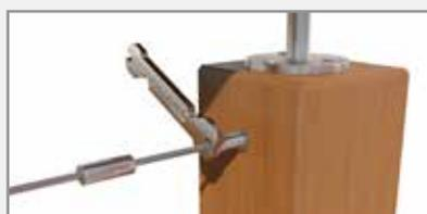
Thread tension rod into the threaded insert and tighten using the ProRig c-spanner until the desired tension is achieved.
