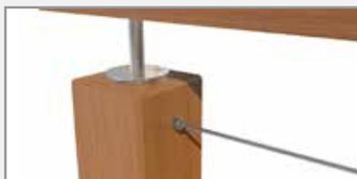
Thread stop bolt end into threaded insert, tighten and lock with PL-10 pliers.
