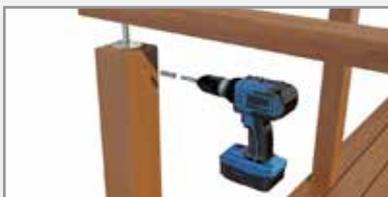
Use the 8mm hex drive bit to screw the threaded insert into the pre-drilled end posts.
