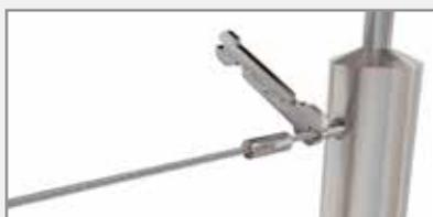
Thread tension rod into the nutsert and tighten using the ProRig c-spanner until the desired tension is achieved.
