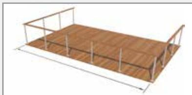
Cut wire 70mm longer than your measured section.
