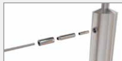
On the open end of the wire thread the finishing cap, tension rod and swage terminal (as above). Crimp the swage terminal four times.
