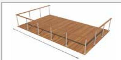
Mark out and drill all posts at the required spacing and hole size (end posts 11mm, intermediate posts 4mm). **Note:** ProRail posts can be supplied with all holes pre-drilled.
