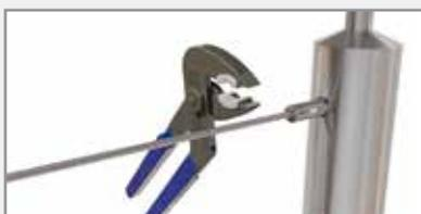
To lock the system in place, tighten the finishing cap against the head of the nut rivet using the PL-10 soft jaw pliers.
